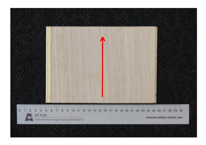
**Figure 1:** GH Engineered Timber - 1900x190x14/3 Arrow indicates direction of testing
