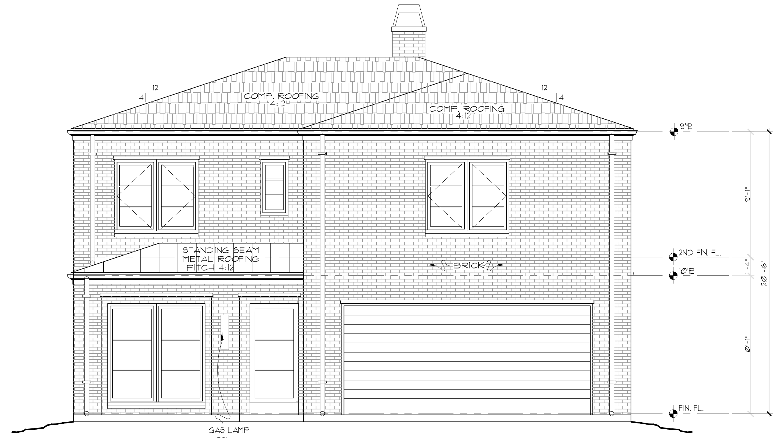
① FRONT ELEVATION SCALE: 1/4"=1'-0"
