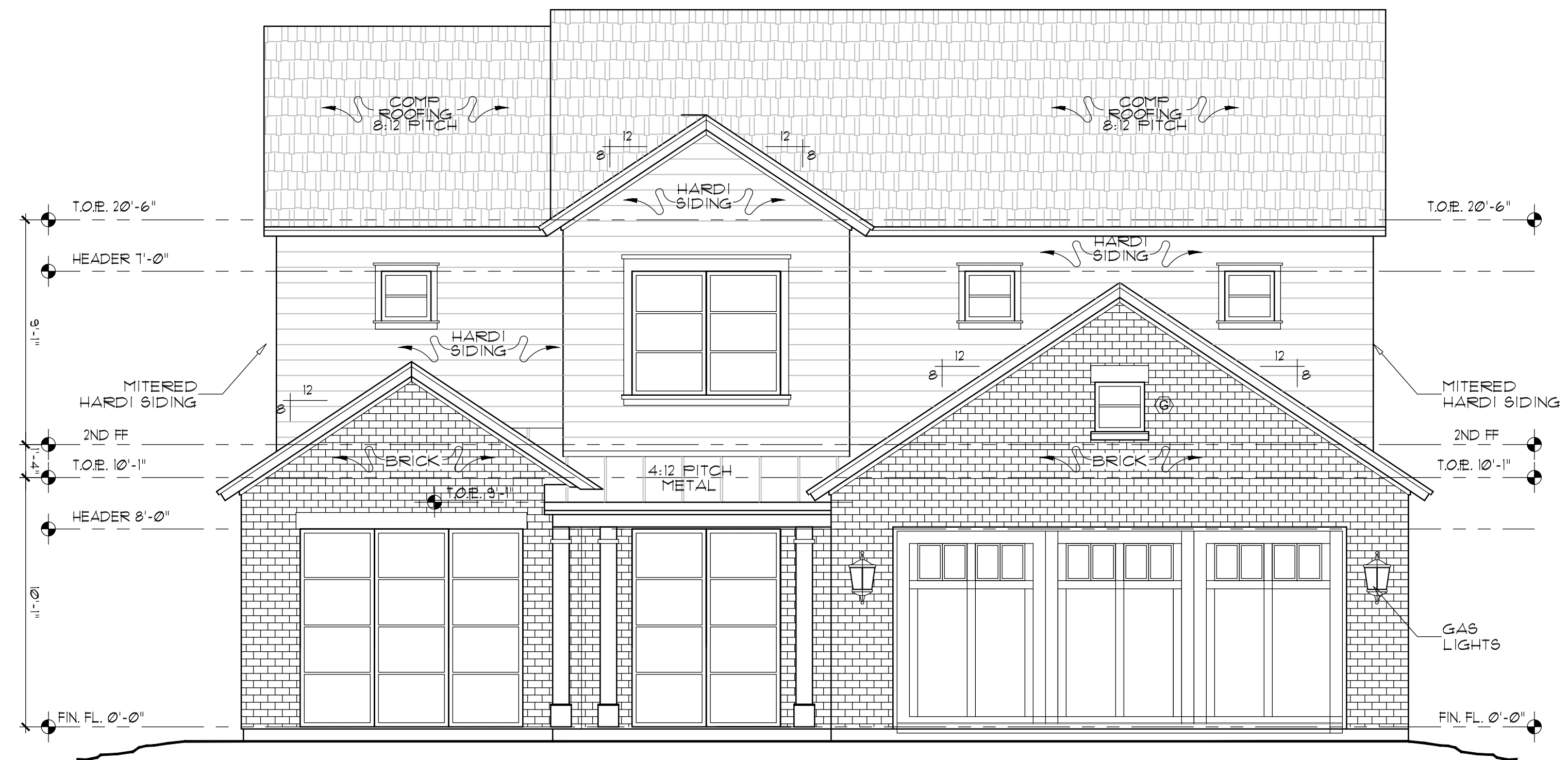
1 FRONT ELEVATION SCALE: 1/4"=1'-0"
