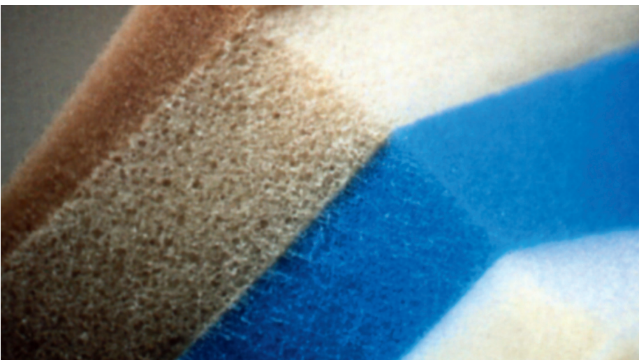
The different colours of the polyurethanes correspond to the different densities.
