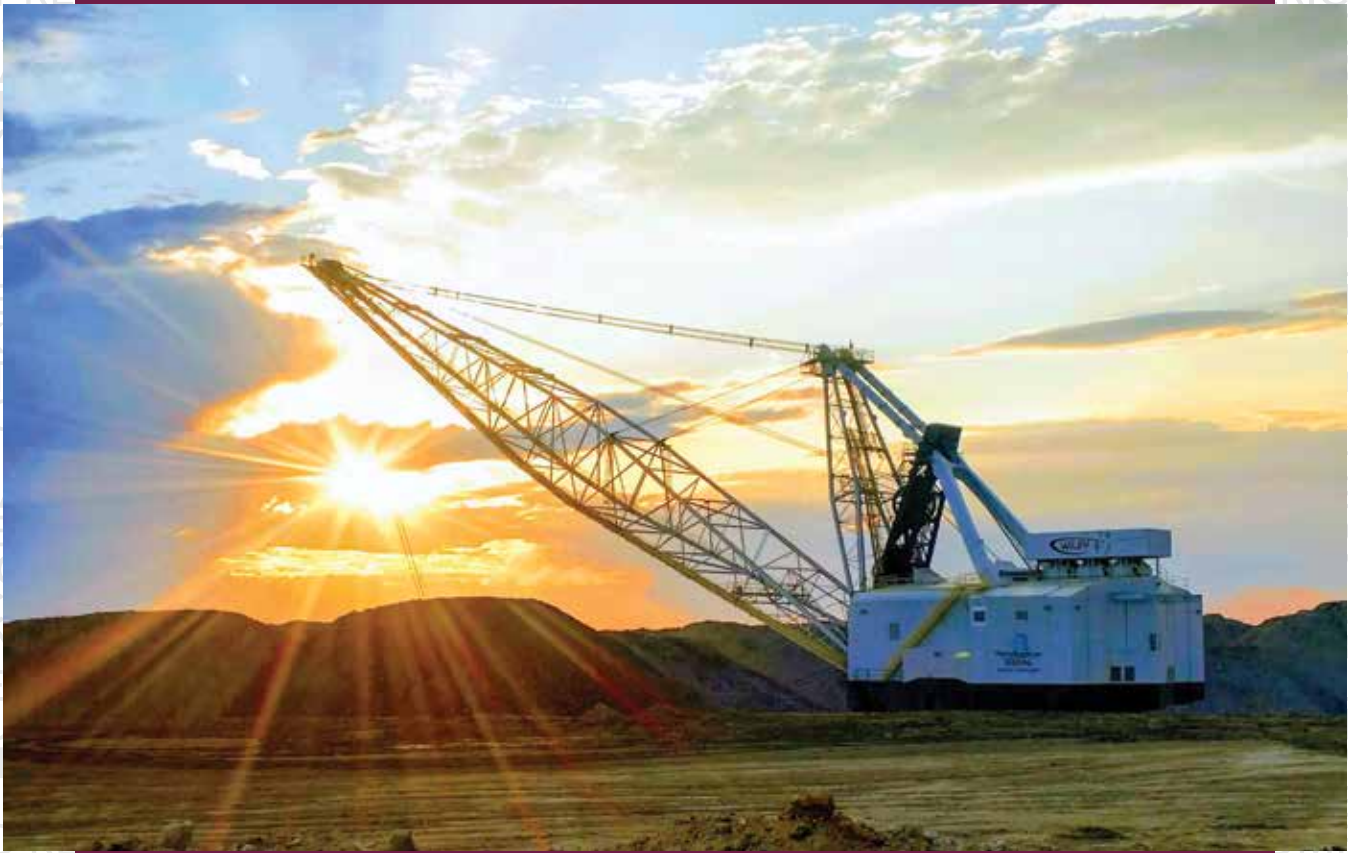
Operating in the early morning sunshine, the Marion 8400 dragline at North American Coal's Coyote Creek Mine near Beulah, North Dakota, removes overburden before the coal below is mined for delivery to the Coyote Station power plant.
