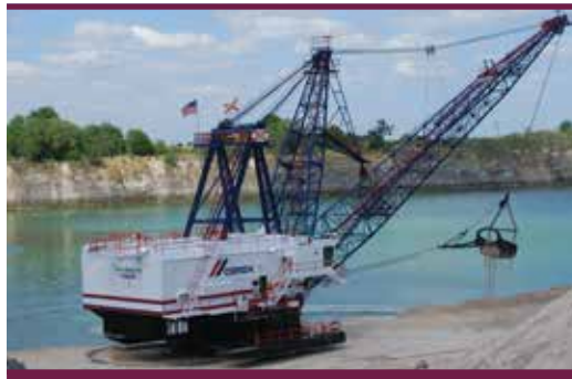
In Sumter County, Florida, a Bucyrus-Erie 770B dragline operated and maintained by North American Mining excavates limestone at the Center Hill quarry owned by CEMEX.
