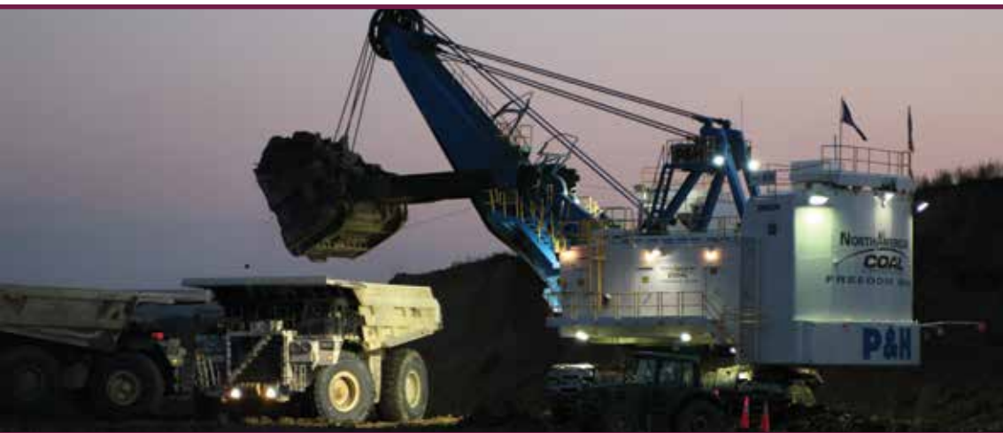
Left: A Kress coal truck at the Falkirk Mine in North Dakota delivers 200 tons of coal to its customer's power plant. The coal will be delivered to the plant via the newly constructed silo feed conveyor pictured in the background. Right: A P&H 2800XP shovel and a fleet of trucks work into the evening at The Coteau Properties Company's Freedom Mine in North Dakota.
