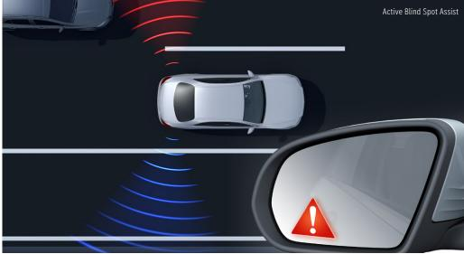
Active Blind Spot Assist can warn the driver of vehicles in the blind spot during a lane change
