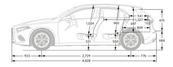
All measurements in millimetres. The dimensions shown are mean values and apply to standard-specification, unladen vehicles
