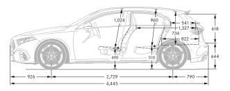
All measurements in millimetres. The dimensions shown are mean values and apply to standard-specification, unladen vehicles
