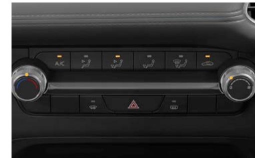
Dual-zone climate control air-conditioning
