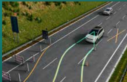
Lane Assist Plus helps the driver stay in lane by subtly adjusting the steering
