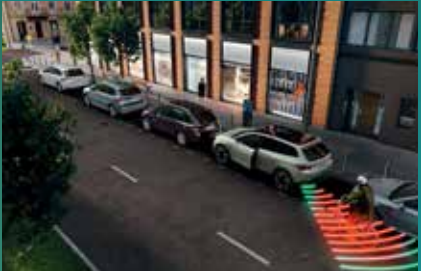
Side Assist – including Exit Warning , Rear Traffic Alert – and rear-view camera monitor the situation behind the vehicle
