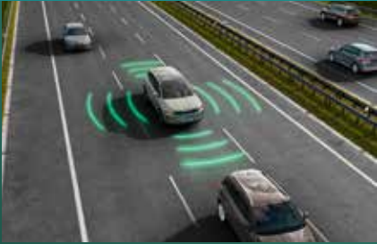
Emergency Assist safely stops the vehicle if the driver fails to respond to warning signals, indicating potential medical emergencies
