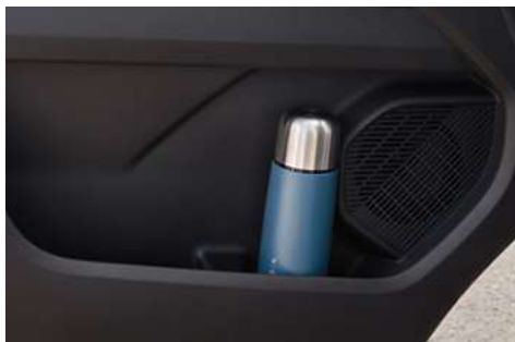
Front door lower storage capacity of 7.5L, with space for 1L bottle
