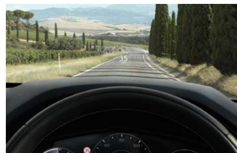
Windscreen projected colour Active Driving Display
