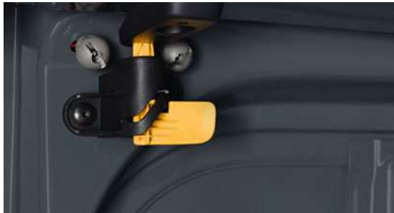
This clever device lets you lock a rear door open
