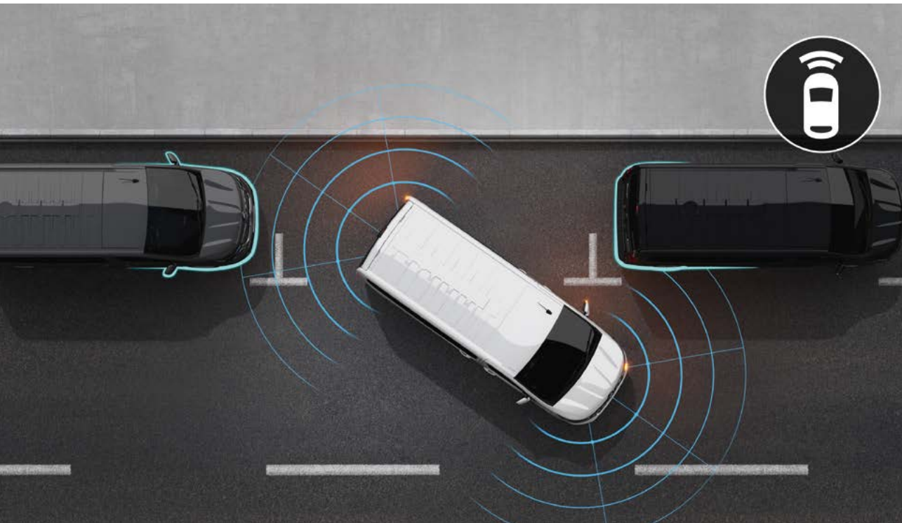
the 360° parking sensors Front, rear and side sensors warn you of objects using an audible and visual signal. You no longer need to worry about damaging your bodywork (Standard on Extra Sport).
