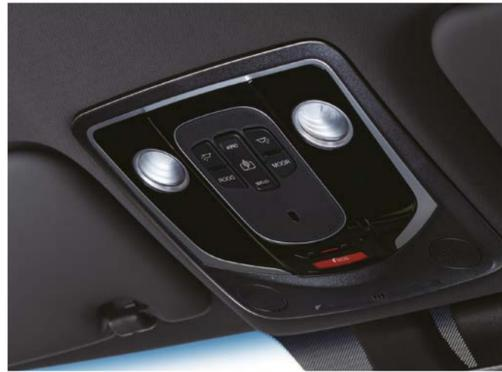
Overhead console with touch-controlled LED cabin lamps
