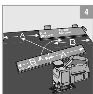
*Begin the next row with the piece left from the previous row (B, min. length 50 cm) (picture 4). Put this piece (begin on the right side) close to the first row – tongue facing groove of first row – lift it in an approx. 30° angle into the groove of the long side, push it down until it fits (picture 1). Should there be any small gaps you might use a tapping lock to knock them gently together to close the joints.*
