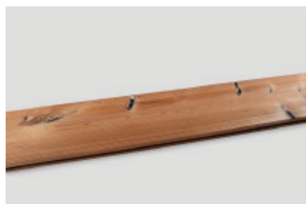
General quality appearance clearly weakened (several knot holes).
