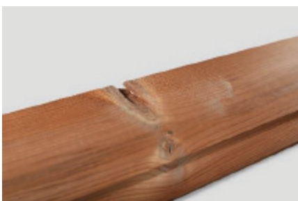
Large crack of a (sound) knot.
