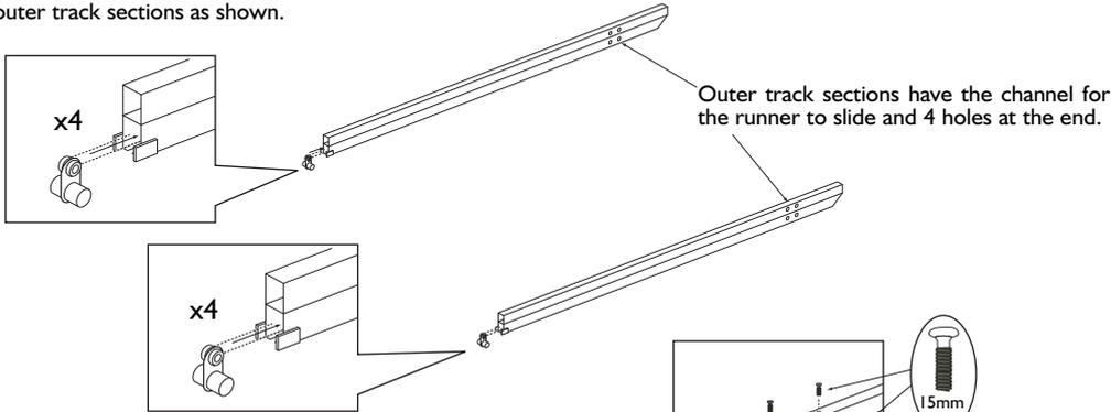
Connect the track sections to the track sections with coupling. Insert the coupling into the upper tube of the track. Secure in place using 4 x 15mm bolts for each join.
