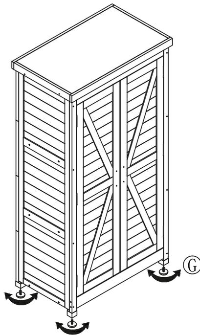
Adjust the plastic feet if necessary.
