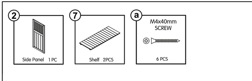
Assembly the Right Side Panel using six **a** Screws
