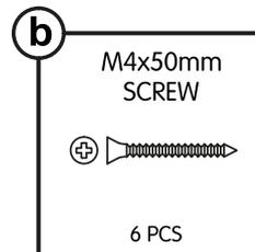
Assembly the Back Door using Six **b** Screws.
