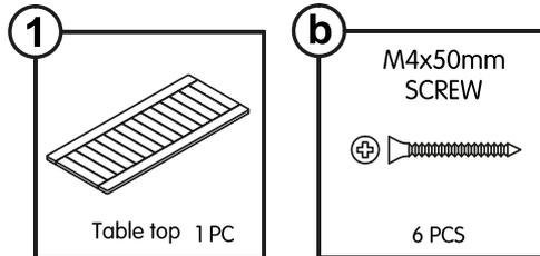
Put the Table Top in Position and Fix Tight using six (b) Screws.
