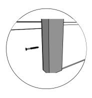
Drive the screw in pre-drilled holes on the frame brackets
