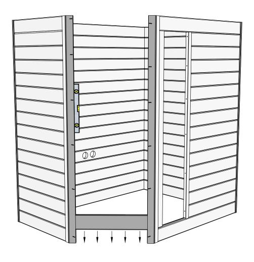
1. Install the door frame brackets (which is cut 45°) in the opening where door frame bracket is.
