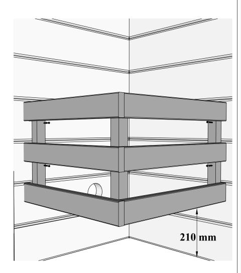
If possible, adjust the height of the heater protection according to the heater purchased. If not use default installation height.
