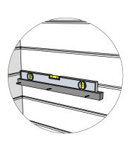
Make sure to level when installing bed holders
