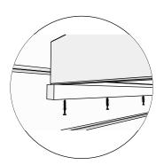
Use screws to fasten sauna bed in pre-drilled holes
