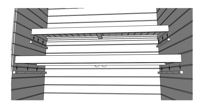
Place the upper sauna bed on the holder and fasten with screws. We recommend to leave the lower sauna bed loose so you can adjust it if needed
