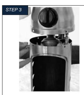
3-1. Put the burner on the tank housing then fix them with 4 pcs 3/16" bolts.
