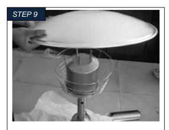
9-1. Put the reflector through the pins and on the washers.
