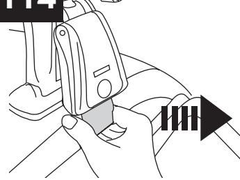
**Caution!** Check clips after installing. Grab each clip and try to pull them away from your vehicle. Pull hard! If the clip moves tighten the adjustment post. If the clip still moves, recheck your measurements between the towers and adjust if necessary. Check clip again.
