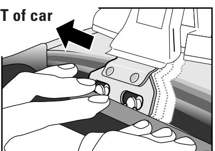
**Remove Rack when not in use to prevent damage to the internal door trim.**
