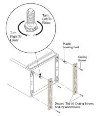
**LEVELING** – You can level your unit with the screw-type adjustable leveling legs on the front corners of the unit. Turn
