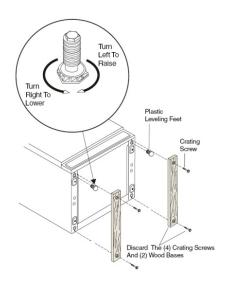
LEVELING — You can level your unit with the screw-type adjustable leveling legs on the front corners of the unit. Turn counterclockwise to raise the corner; turn clockwise to lower it. Leveling legs are required in front only. Unit may have a slight tilt from front to back after legs are installed. This is acceptable and is recommended on this unit.
