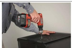
3. Remove the bracket and use a ¼" drill bit to drill the 4 holes you marked on top of the refrigerator.
