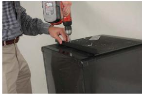
5. Place the bracket on the refrigerator. Secure the bracket by fastening the flat head screws through the bracket and into the plastic anchors.
