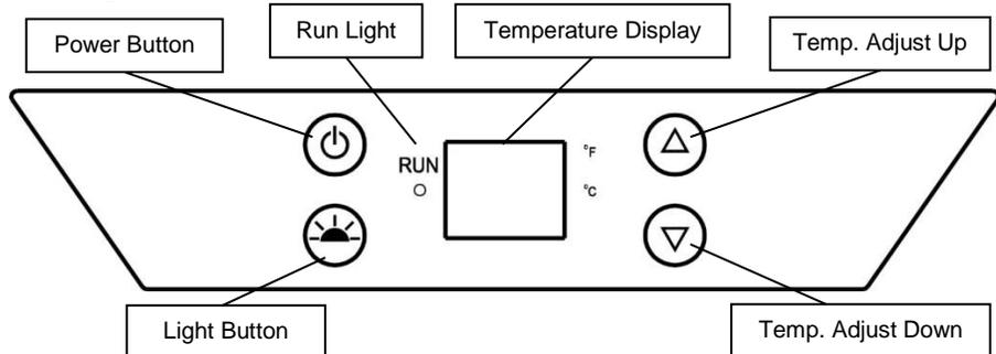
Use the up and down buttons to adjust the temperature. The temperature displayed can be in Fahrenheit or Celsius. This precision refrigerator has a temperature range from 32°F to 50°F.
