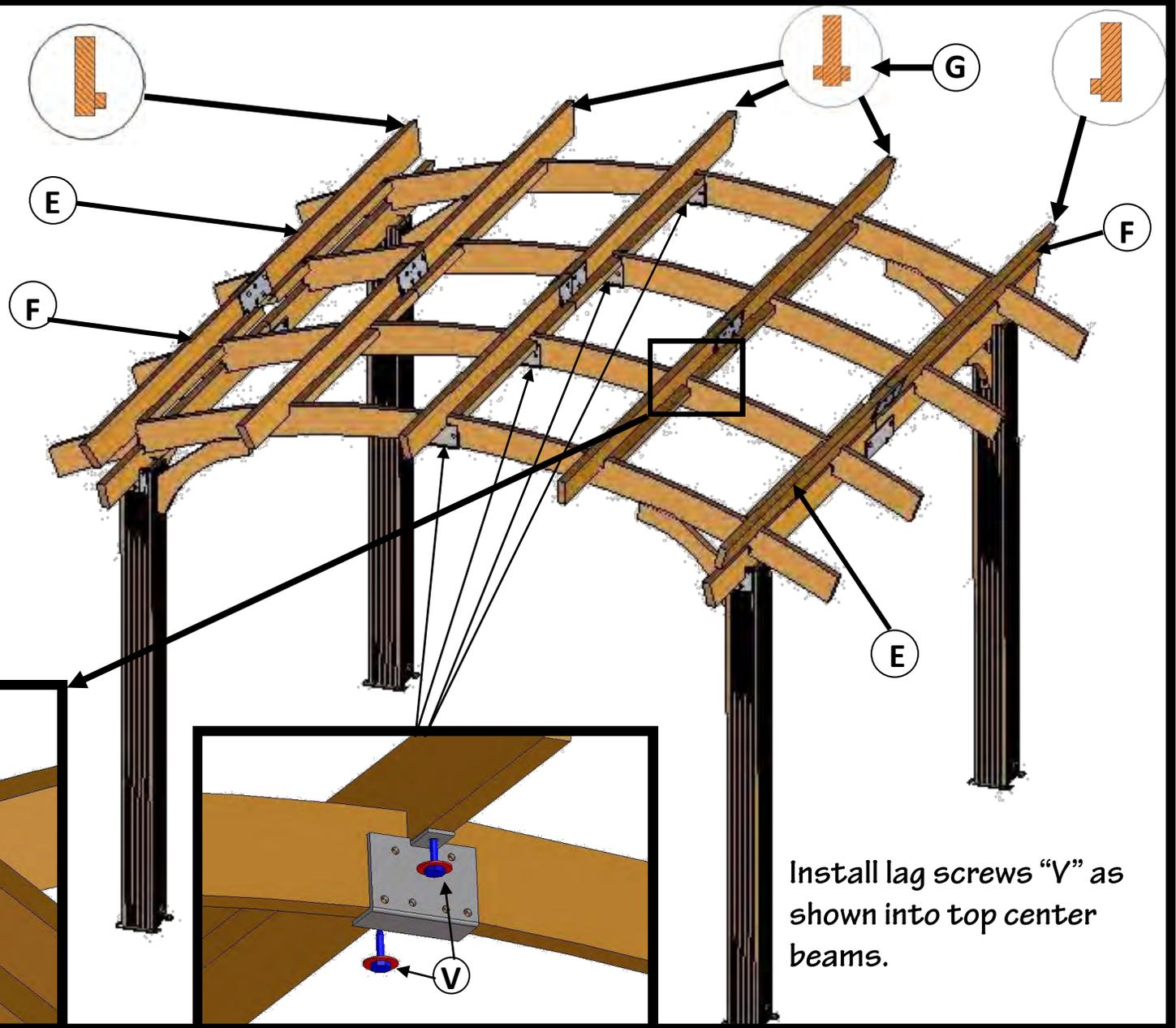
Install lag screws "V" as shown into top center beams.
