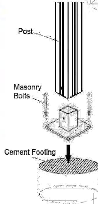
(Suggested for installation on lawns. For other surfaces, appropriate mounting methods should be used.)
