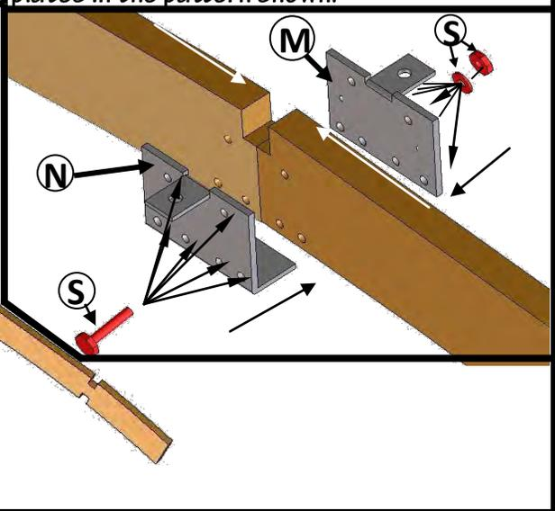
**NOTE:** In the remaining steps, a rubber mallet may be useful in fitting beams together properly.
