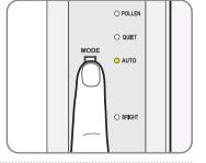
Sleep Mode Indicator turns on in Silent Mode, which automatically switches off Mood Light and Air Quality Indicator.
