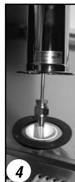
Thread beer line connector to draft arm and secure draft arm to cabinet with rubber gasket under the draft arm.
