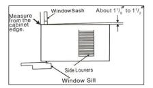
3. Check that the air conditioner cabinet is tilted back about 1 ½", which should be about 3-4 degrees downward to the outside. After proper installation, condensation should not drain from the overflow drain hole during normal use, correct slope or otherwise.
