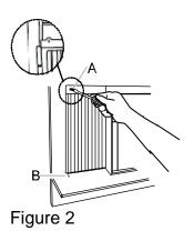
A. #10 x 3/4" Flat Screw B. Slotted hole in the bottom of the curtain
