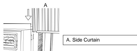
5. Insert the top of the right-hand curtain housing to the top curtain channel as shown below:
