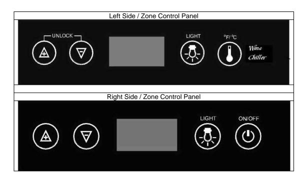
You can select temperature display setting from Fahrenheit to Celsius degree by pushing the °F/°C button/mark. Fahrenheit or Celsius degrees indicator will appear in blue color in the temperature display window for each zone.
