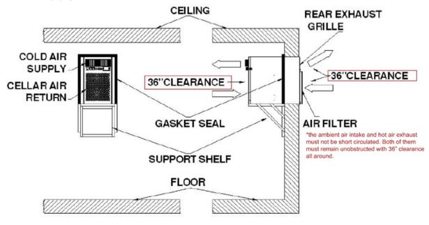
Flush to the outside of wall with air filter & rear exhaust grille
