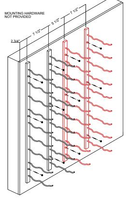
3 - Determine appropriate fasteners for the wall surface and fasten the strips to the wall.
