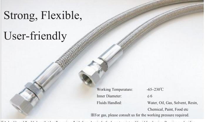
\*A durable and flexible hose that handles various fluids from chemicals, food, gas to paint and liquid for cleaning. By using our braiding technology, this hose is reinforced with high strength fiber and stainless steel wire which leads to high pressure resistance and high strength towards bending.
