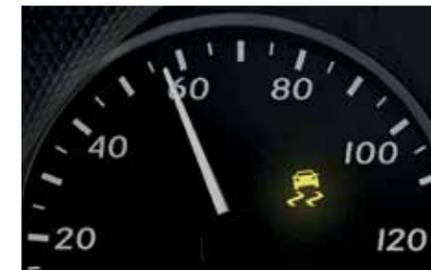
**Load-Adaptive Electronic Stability Program (ESP<sup>®</sup>)<sup>3</sup>** This dynamic handling system actively intervenes to help keep the van firmly under control and safe by automatically braking individual wheels and reducing engine power to help stabilize the vehicle if wheelspin, understeer, or oversteer is detected.
