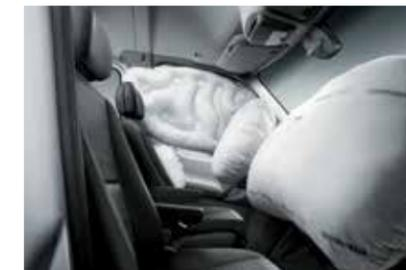
**Driver and Passenger Airbags<sup>7</sup>** The driver and passenger front, thorax, and window airbags<sup>7</sup> help protect you and your passengers in the event of a collision.
