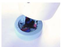
Heat the scraps with the heat gun until it is softened.
