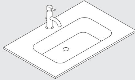
7. Spread non-acetic silicone sparingly along top rim of vanity. Position sink in place and use a cloth to wipe excess silicone.
