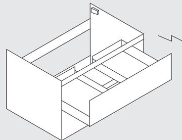
4. Hook vanity onto wall brackets. Mount support bracket onto wall directly under vanity base.
