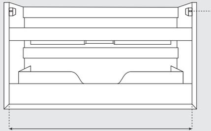
2. Drill mounting holes in wall and fasten wall brackets with screws.
