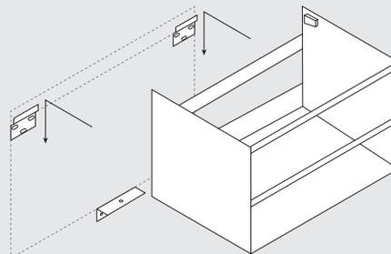
5. Adjust metal hooks if necessary to properly level vanity and secure it to wall.
