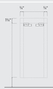
3. Drill mounting holes in wall and fasten wall brackets with screws.
