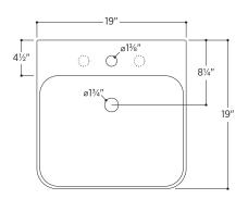
All measurements are approximate and for comparison only. Please note that these dimensions and specifications are subject to change without notice. Our products must be installed by certified professionals only and according to our installation guide, as well as federal, provincial/state and local building codes and regulations.
