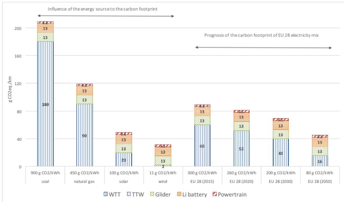
Figure 8: GHG emissions of electric vehicles depending on the energy sources and the prognosis of the reduction in carbon intensity. Electricity based on [21]
