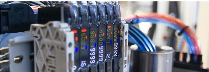
From photoelectric and capacitive sensors to detect boxes and plastics; limit switches and position sensors as well as vision sensors and barcode scanner to ensure packaging is complete and correctly marked.
