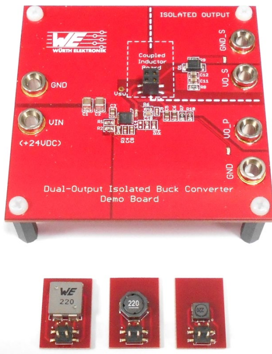
Figure 65: Buck converter with isolated output Evalboard with WE coupled inductor plug-in boards Detail
