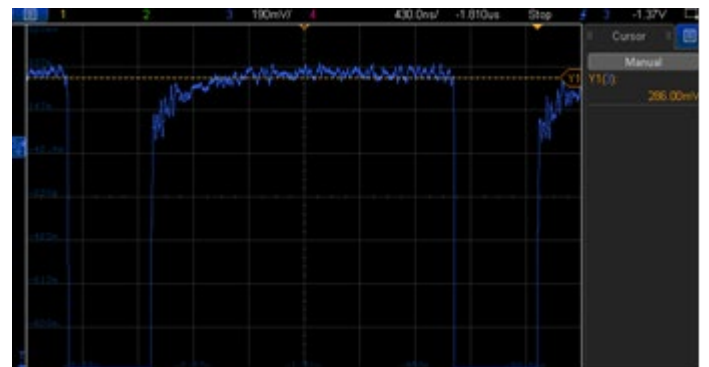
Figure 30: Experimental result for Diode average forward voltage drop during off-time
