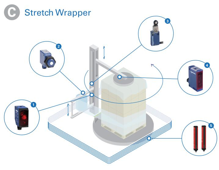
1 XUK Laser Photoelectric Sensor Distance measurement to the pallet.
