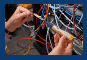
Quickly verify fiber activity, polarity, and connectivity with the FiberLert™ Live Fiber Detector. No setup or interpretation required.
