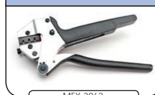
Hand Tool, Stamped & Formed Contact, Size 16, 20-14 AWG
