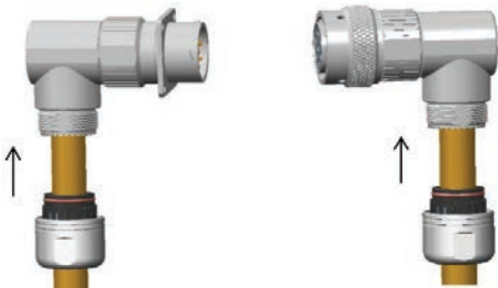
Step 11: Push shielding clip into backshell
