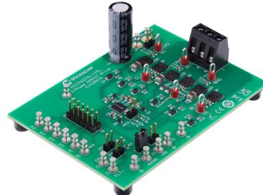
The MIC4607A MOSFET Driver Evaluation Board is a MOSFET controller for driving Brushless DC (BLDC) motors. The input voltage range for the MOSFET bridge is  $-0.3\text{V}$  to  $+85\text{V}$  and the input voltage range for MIC4607A is  $5.25\text{V}$  to  $16\text{V}$ . It is a versatile, two-layered, low-cost, high-current and easily configurable board. Several key test points are available on the board in order to facilitate the user's measurements, tuning and motor control optimization.
