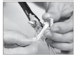
6.2 Position the lock cap from behind onto the extension bracket while capturing either the dielectric or metallic strain members.
