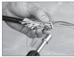
6.3 Making sure that all parts of the connector are kept in alignment, proceed to tighten the lower securing nut completely. Torque nut to 30-35 in-lbs (3.4-4.0 kg·m).
