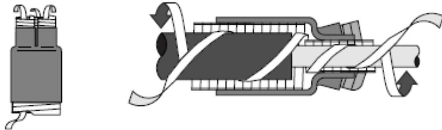
2. After measuring required length, install RJS – Series silicone rubber phase re-jacketing sleeves.
