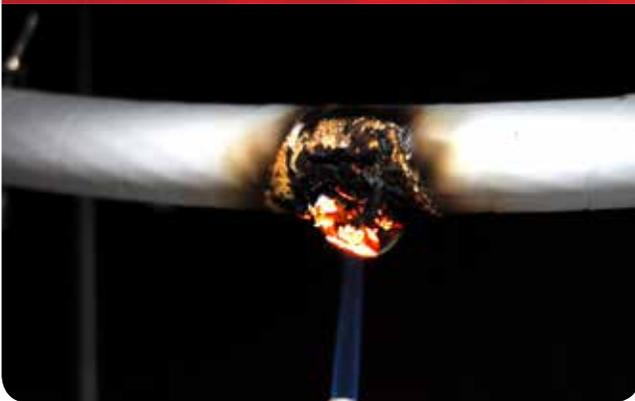
Cable Protected with Scotch® Tape 77 After Test
