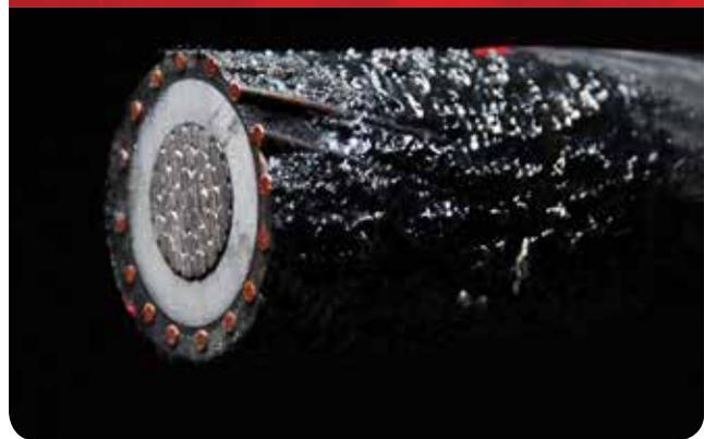
Cable Protected with Scotch® Tape 77 During Test
